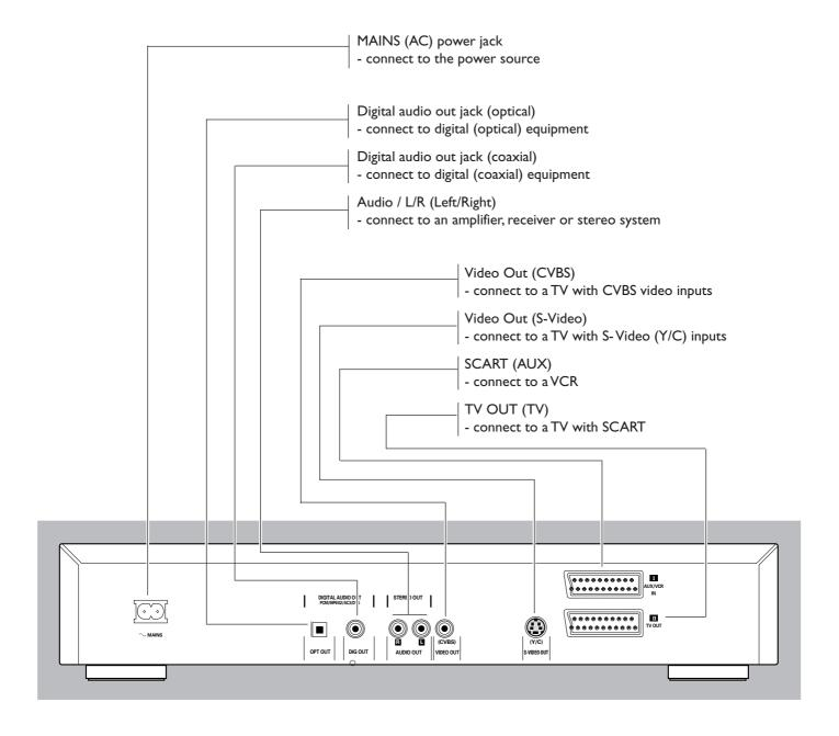
Caution: Do not touch the inner pins of the jacks on the rear panel connectors. Electrostatic discharge may cause permanent damage to the unit.
